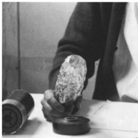
**Fig. 9.12.** Wrap scintillator loosely in aluminium foil
