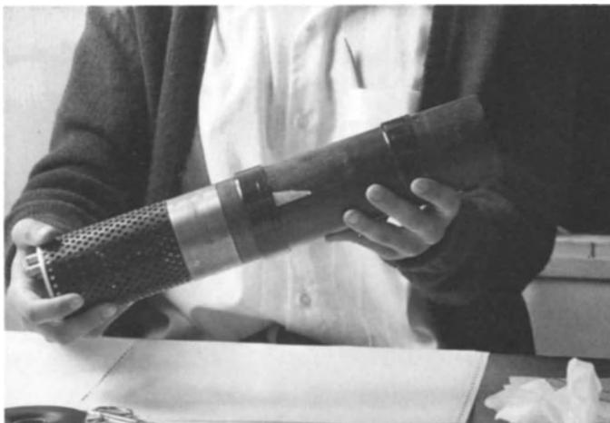
**Fig. 9.14.** Assembled scintillation detector
