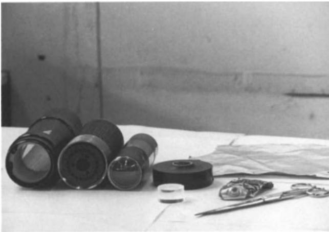
**Fig. 9.10.** Materials for mounting the scintillation detector
